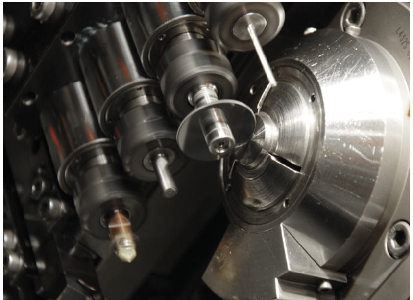
Ti-Loc In-Machine Slitting Saw
